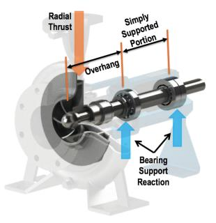
overhang length reduces the bending moment, the life of the bearing is further enhanced. With higher radial thrust handling capability, the vibrations of the pump are contained and the probable mechanical damage if the pump operates near to shut off (highest pressure point) is also reduced.
